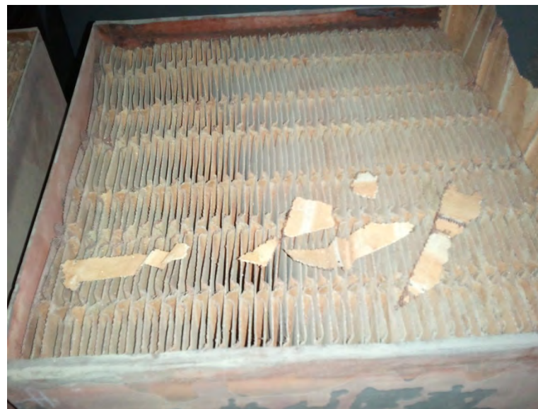
Hand Torn Pieces from Element Pulled Up on Right
