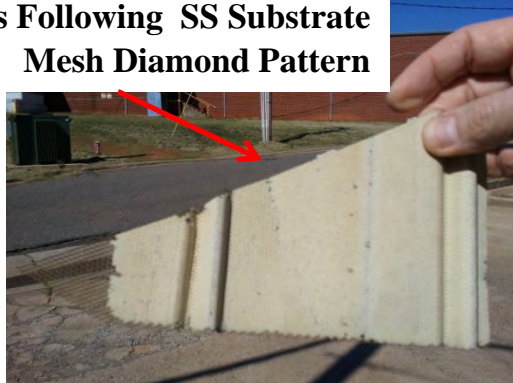
Plate Catalyst With Type 400 SS Mesh Substrate Material With Visible Corrosion Increasing Aged Catalyst SO 2 to SO 3 Conversion Rate (Test A to Test B Consideration)
